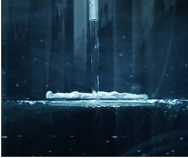
FIG. 1. A side view of a metal disk floating just below the surface of the water, with a boundary jump occurring at the edge of the disk. The photograph was taken in a transparent cylindrical vessel for demonstration purposes only. Due to a lensing effect caused by the vessel, the disk appears larger than the surface disturbance. A video capturing this phenomenon can be viewed in [8].
